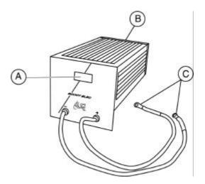
Instructions for use: Disconnect and remove the 3 cells Connect the cell to the discharge bench - Red wire to the cell + terminal - Blue wire to the cell - terminal Tighten the terminals, the cell voltage is displayed The cooling fan (B) runs (if the voltage is between 7.5 V and 4.5 V) The cell discharges automatically When discharge is finished, the fan stops and the discharge time is displayed in minutes on the display (A) (e.g.: T=50)
