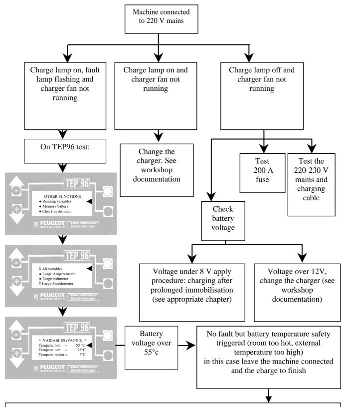
If after 2 hrs the battery temperature is not under 55°, check the battery temperature functions and change it if necessary (sensor fault, or sensor information error).
