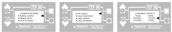
The DISCHARGE value must be between 0 and 110 Ah
