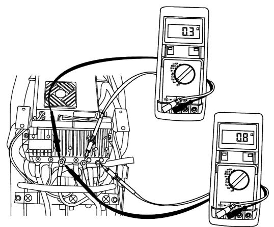
If the resistances are not correct, the motor and the ECU must be changed.
