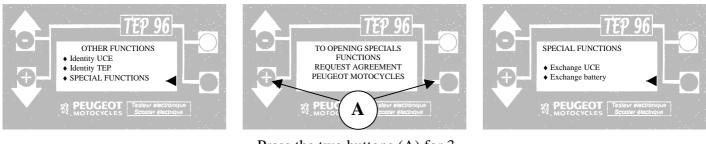
Press the two buttons (A) for 3 seconds
