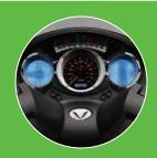
**Instrumentation:** Vital functions are shown in a high-tech display, with system status on the left, battery charge on the right, and an analog speedometer placed front and center.
