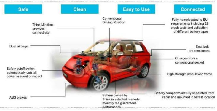
Purpose-built EV platform designed to volume auto OEM standards
