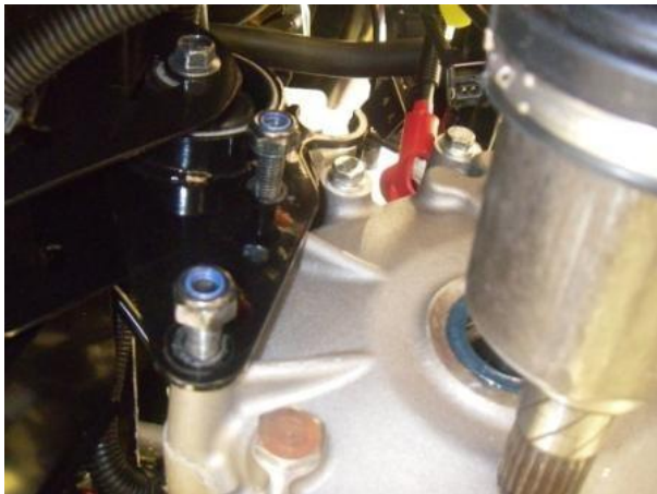
Rear motor bracket (on the gearbox)
